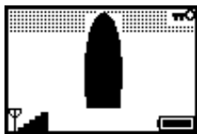
AA710 System locked. Hold Mode button to clear.
